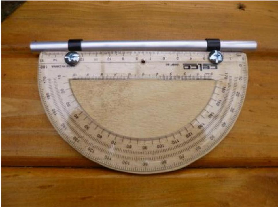
*Protractor, backing board with sighting tube attached*
