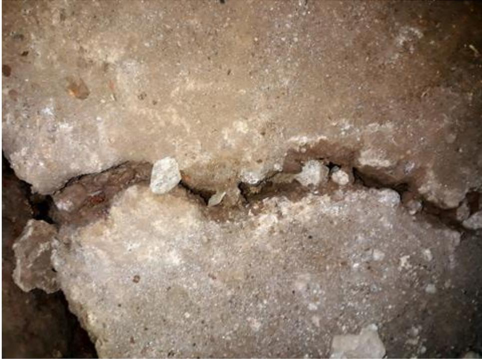
*Our soil has a high clay content, and it cracks pretty dramatically when drying out*
