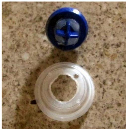
*Inlet valve head seal - the old one, showing that the seal has come completely off the support fitting.*
