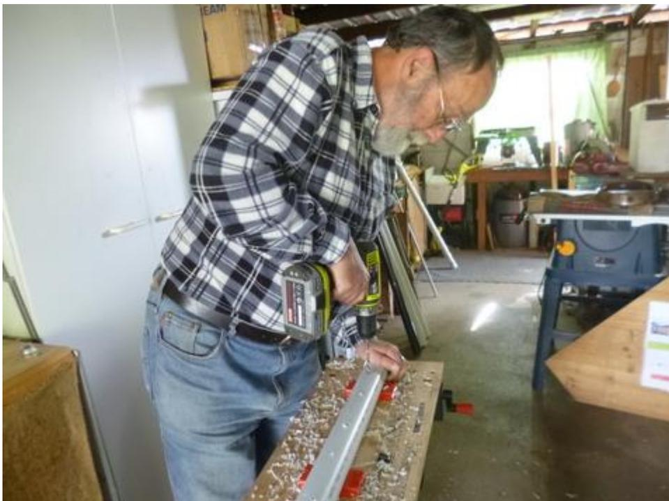
With the holes in place in two of the one metre lengths I glued an end cap on one end and a 90° elbow onto the other of each one, using the blue PVC plumber's glue. I then cut the third one metre length of 50mm pipe in half and slid half into the other side of
