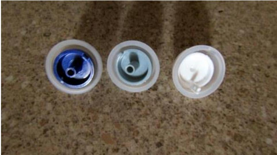
**Left:** original seal **Centre:** new replacement seal (correct) **Right:** New seal which Ilok OK from the front but rear was totally different
