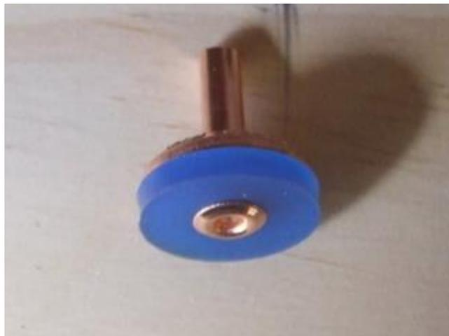
*New style washer stem showing attachment rivet*
