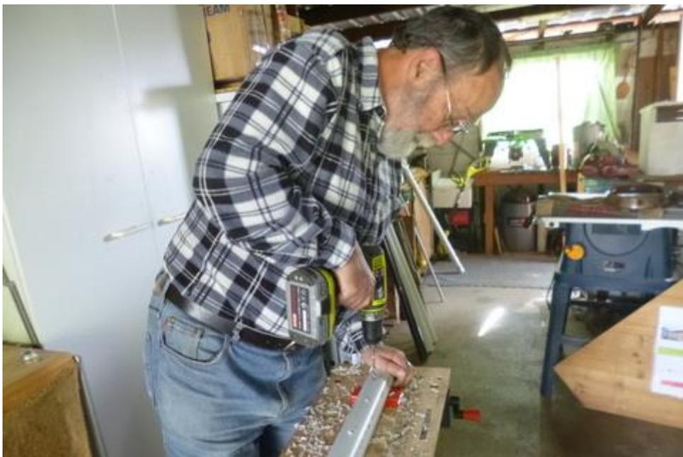
With the holes in place in two of the one metre lengths I glued an end cap on one end and a 90° elbow onto the other of each one, using the blue PVC plumber's glue. I then cut the third one metre length of 50mm pipe in half and slid half into the other side of the 90° elbow giving two L-shaped sections. The idea was that the pipe with the holes would sit along the bottom of the tub horizontally and water would flow in through the vertical section of pipe.
