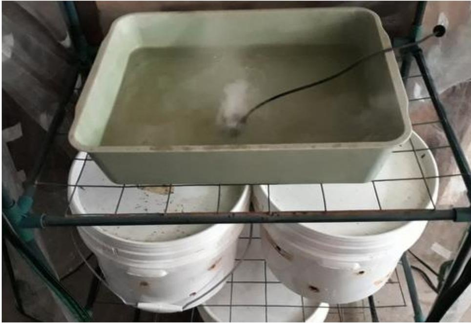
I got hold of a fogger/mist maker of the type used in small indoor water features, you know, the ones with a fountain that is shrouded in mist for a calming effect. You plug the fogger in and immerse it in a water supply, it uses ultrasonic waves to create a mist which then rolls out over the fountains landscape.
