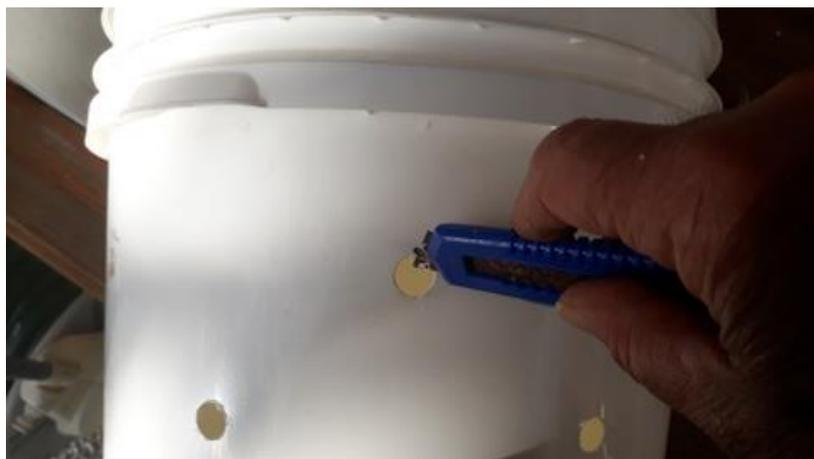
*Main hole drilled and being deburred*
