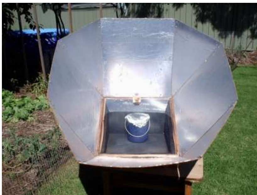
The aluminium foil – not as reflective as it once was
