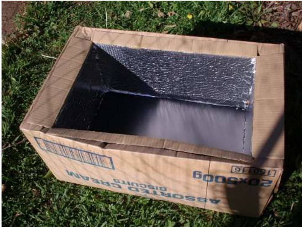
Inside the inner box showing alfoil lining and matt black metal plate
