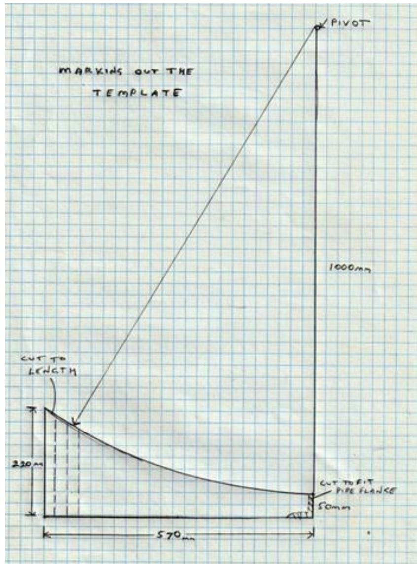
With the rib set out, cut it along the lines with a knife, saw or if you have one, a band saw, making sure to stick exactly to the line. If all else fails cut the rib out a bit larger than the line, then use sandpaper to remove the material outside the line. Obviously, the more accurate the template is, the better all the ribs will be. There will also need to be a cut out from the bottom of the low end so that it can be fitted over the pipe flange in the centre of the baseboard.
