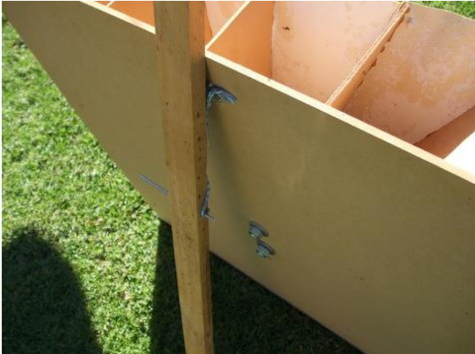
To use the support it is just a case of hooking the twine over the cleat and then around the aluminium welding rod through the pine support. The angle can be varied by moving the aluminium rod through a higher or lower hole, depending on the angle of the sun.
