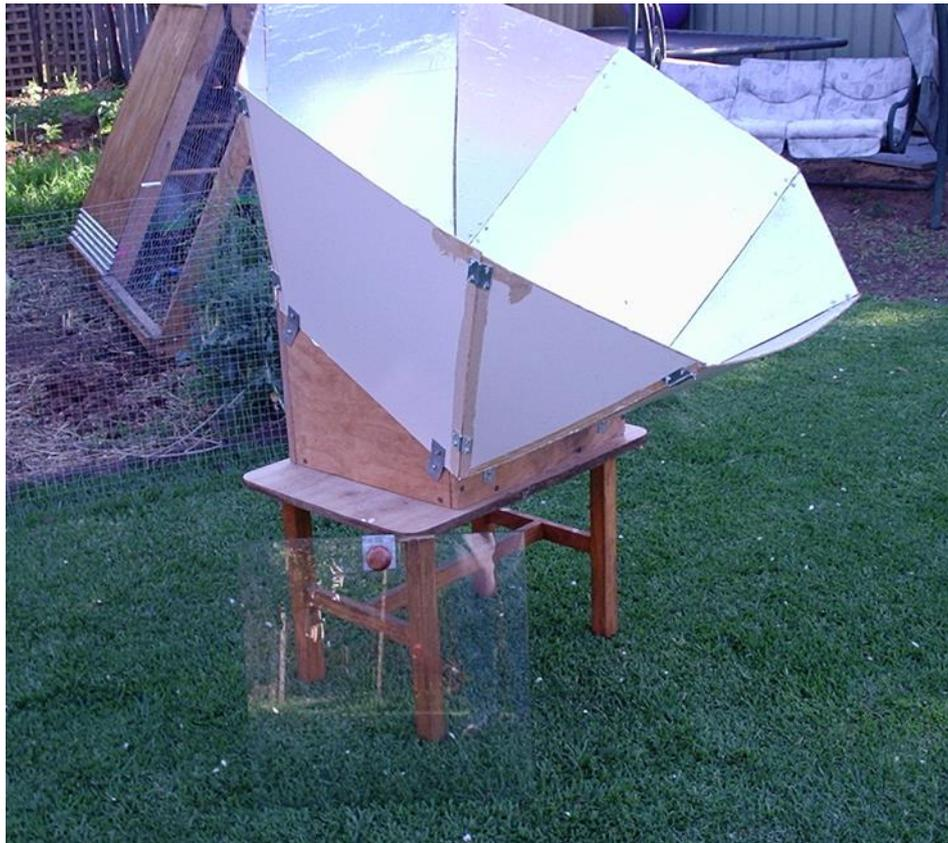
The oven, once assembled, takes up a lot of space, and unless you have large amounts of free space (which we don't) it is handy to be able to separate and flatten out the reflector into sections for storage. As my elder daughter's boyfriend asked when he went out into the backyard and saw the completed solar oven – "Wow! What are you doing with the satellite dish?"
