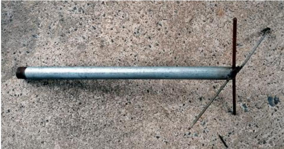
I made a mark around the pipe where the focal point was (quickly! It heated up remarkably fast!) then turned the cooker out of the sun. When the pipe had cooled I traced around the pipe at the focal point parallel to the ground, removed and then cut the end of the pipe off with my angle grinder. That way the end of the pipe would be flat when I wanted to put anything on it.
