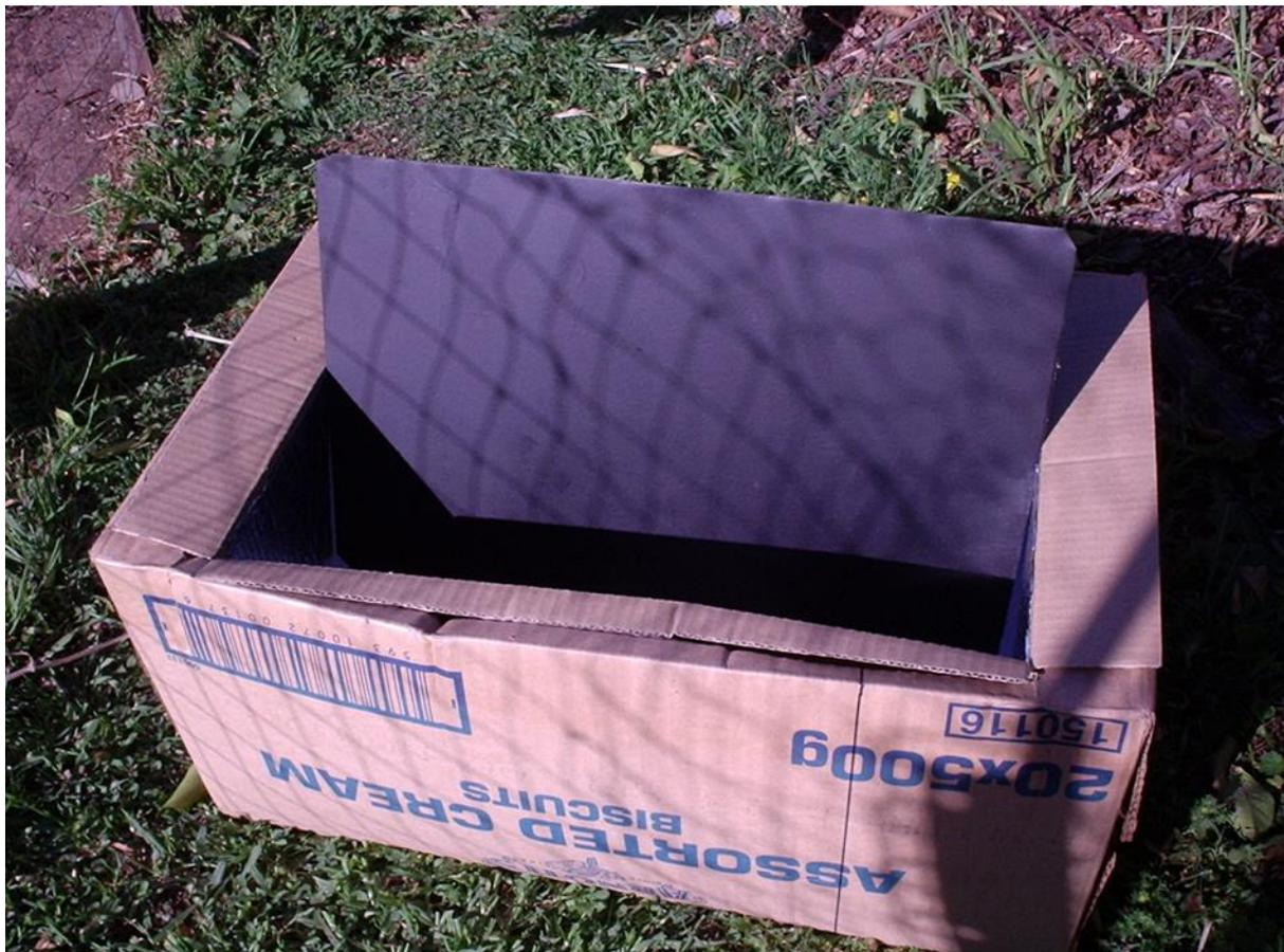
Well, I put in a matt black steel panel and believe it or not, it did! All of a sudden I could get up to 90°C and was able to cook an aluminium billy full of spuds perfectly in less than two hours. This technology made sense and worked fine if you set it up right.
