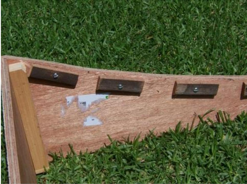
To put the mirrors in I screwed supports made from 20mm x 5mm rounded edge moulding with one side sawn off to make it flat, to the inside of the sides of the reflector box so that the mirror could be put in place inside the reflector box and at the correct angle. Once the mirrors were in place I secured them by screwing more 20mm x 5mm rounded edge moulding along over the top of the ends of the mirrors.
