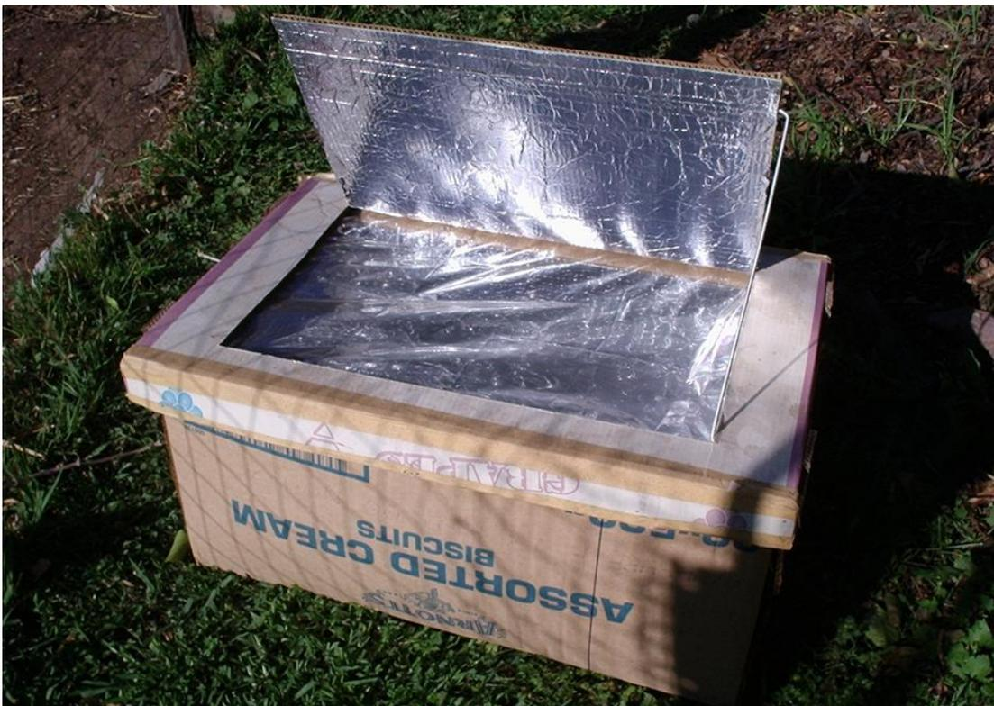
7. The bottom of the flap should also be lined with aluminium foil to act as a mirror to reflect sunlight into the oven. A Z-shaped piece of wire is then inserted in the
