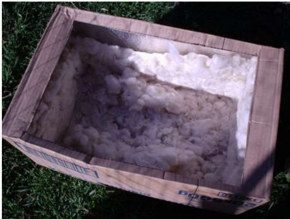
Inside the outer box showing alfoil lining and wool used as insulation
