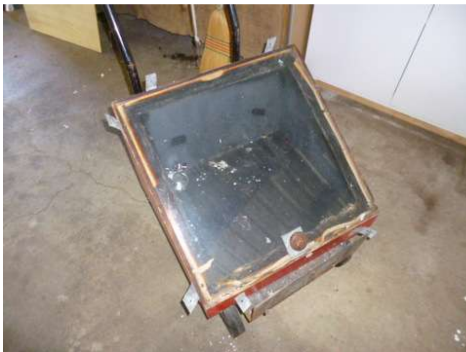
The carcase of the oven with reflector attachments in place
